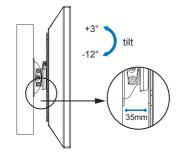
Apply the TV with wall mount to the wall plate
