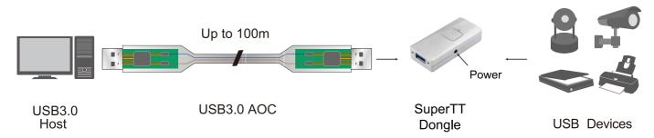
\*USB 3.0 Active Optical Cable is only backward compatible with USB 2.0 when connected with SuperTT Dongle
